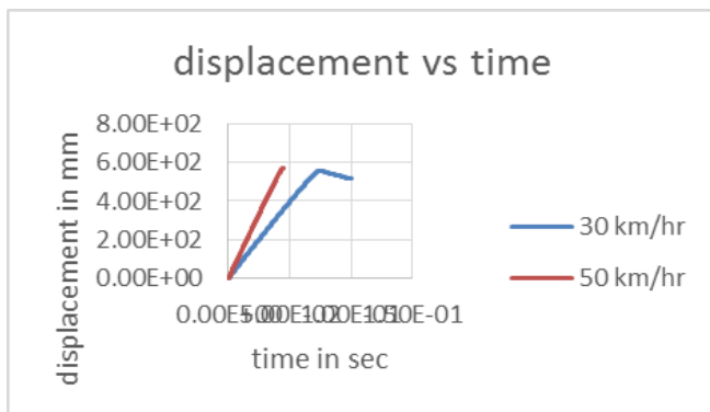
Fig 6 Displacement graph for different velocities of 1200 kg mass
